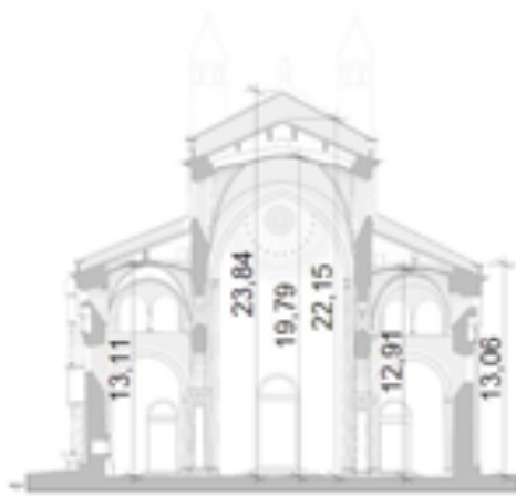
Figure 2. a) A 3D view of the Modena Cathedral (Google Earth); b) Cross-section of the Cathedral of Modena
