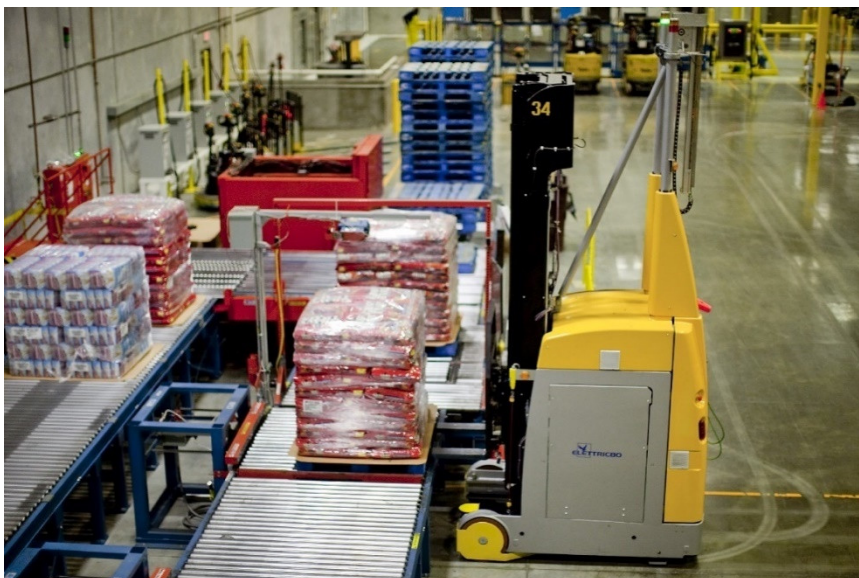
Figure 13 An operating LGV machine
