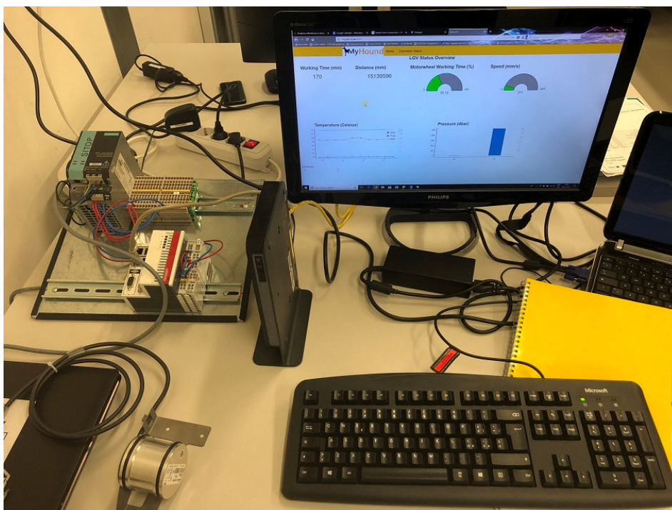
Figure 22 The workbench and a pc used for developing the first release of the software solution
