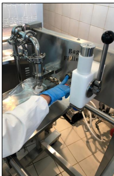
Fig. 56: Start filling bag.
