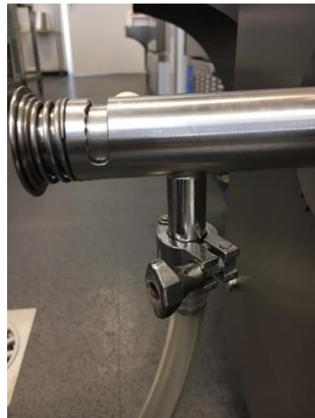
Fig.39: Pastomaster 60 RTL extraction tap connected to extraction tube.
