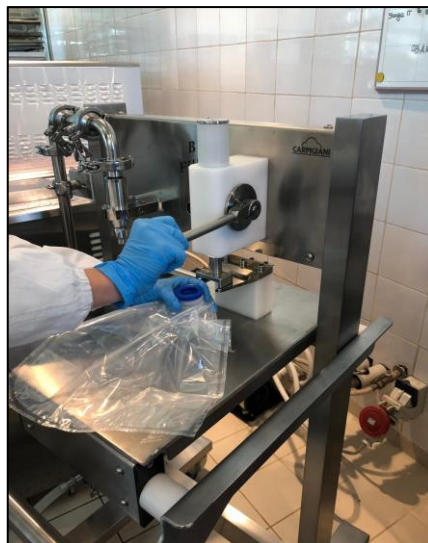
Fig. 54: Empty bag placement.
