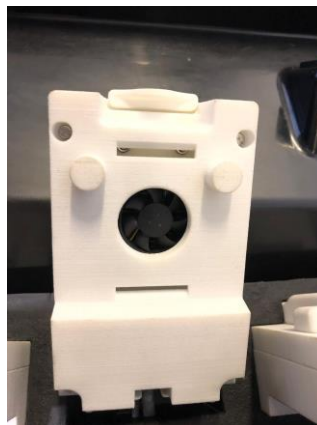
Fig. 20: The Peltier Cell assembled on the measuring chamber.
