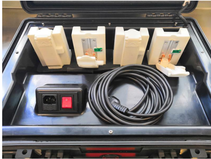
Fig. 23: Thermal chamber in the lower part of the suitcase.
