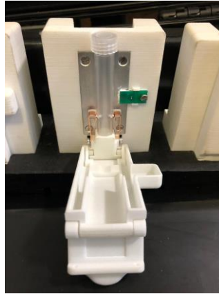
Fig. 19: Test tube in position in the thermal chamber.
