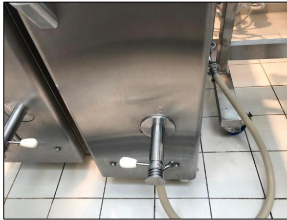
Fig. 53: Pastomaster 60 RTL extraction tap in open position.
