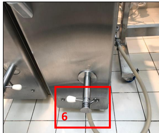
Fig. 52: Extraction tap connected to the bag filling transport tube.
