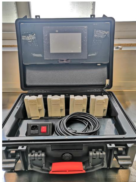
Fig. 22: Touch screen display in the upper part of the suitcase.
