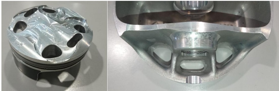
Figure 4.17. Piston top holes machining detail.
