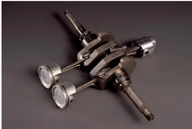
Figure 5.4. Yamaha T-max crank mechanism and balancing system.
