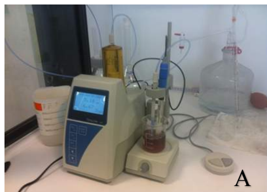
Fig. 4. Basic devices for fermentation monitoring: A. Automatic titrator TitroLine easy; B. Malligand ebulliometer.
