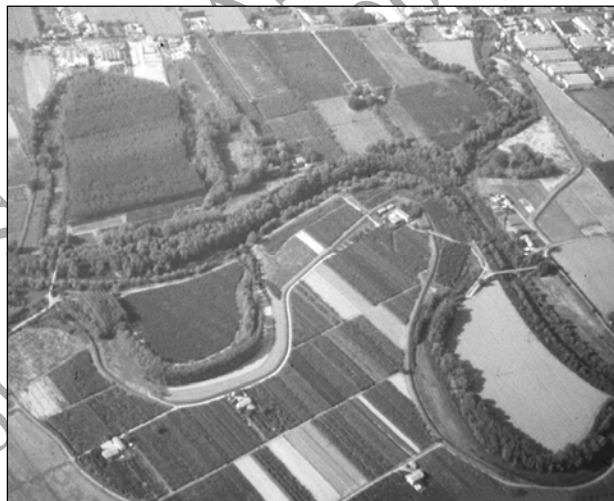
Fig. 7. River Panaro east of Modena that flows from the left (south) to the right (north). The meander cut-offs carried out in the early 1970s are evident
