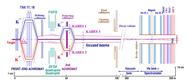
Figure 1: Schematic lateral view of the NA48/2 beam line (TAX17,18: motorized beam dump/collimators used to select the momentum of the  $K^+$  and  $K^-$  beams; FDFD/DFDF: focusing set of quadrupoles, KABES1–3: kaon beam spectrometer stations), decay volume and detector (DCH1–4: drift chambers, HOD: hodoscope, LKr: EM calorimeter, HAC: hadron calorimeter, MUV: muon veto). Note that the vertical scales are different in the two parts of the figure.
