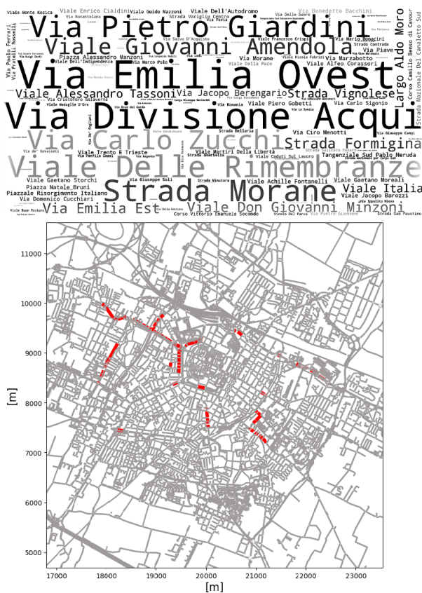
Fig. 7. Word cloud image of the streets whose lane density was above the value of 100 vehicles/km at least one time in the 19th November 2018 simulation between 05:00 and 23:59. The font dimension is proportional to the times in which the lane density value overcome the cut off during the simulation. The red coloured segments in the map are the 100 most congested roads.
