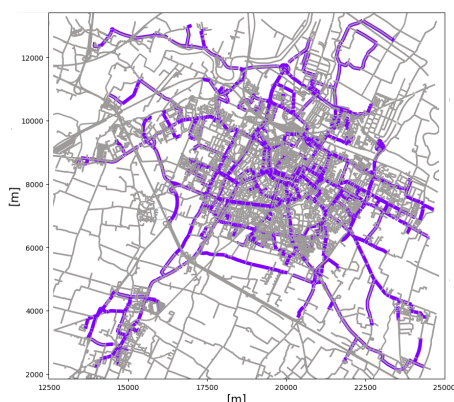
Figure 4: Simulated area with roads that have a significant number of vehicles (above 1000 veh/day) colored in purple.
