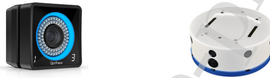
Figure 5: One of four OptiTrack Prime 13 cameras and one of eight K-Team's Khepera IV robots ( \phi = 14.0\text{ cm} , h = 6.0\text{ cm} ) used for the experimental setup in Section 7.
