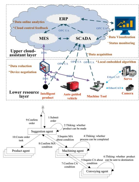
Agent-based fault tolerant framework for manufacturing process automation (Zubair H et al)
