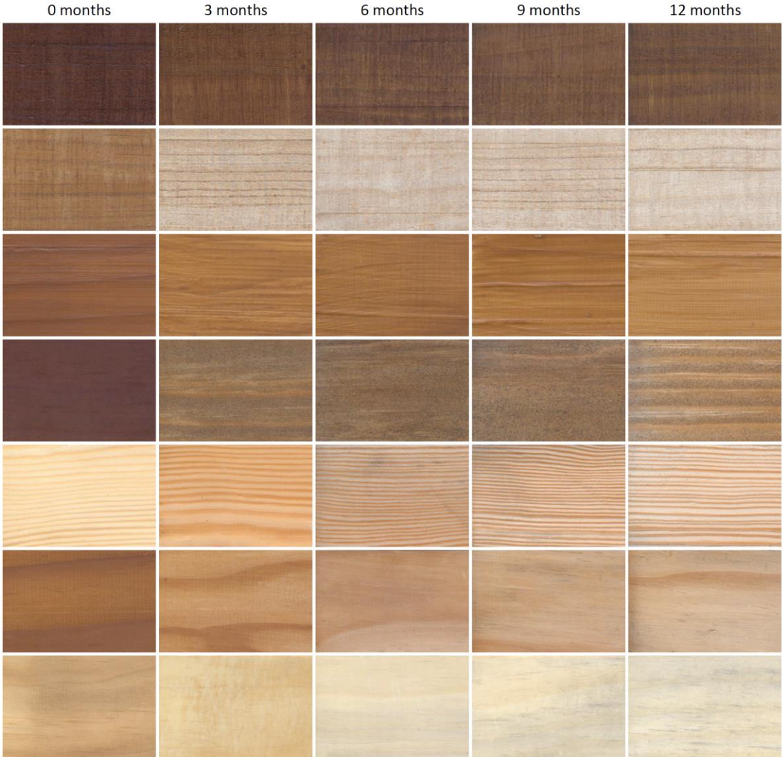
Figure 5: Change of samples appearance along one year of natural weathering (from up: #1, #2, #3, #4, #5, #6, #7).
