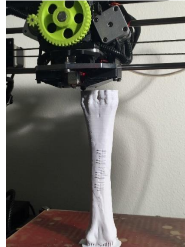
Fig. 3. 3D printing ancient bison metapodial with Lulzbot Taz 5.
