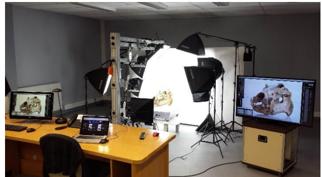
Fig. 2. Photo 3D set up showing the image capture of a hippopotamus skull issued from the zoology collection.
