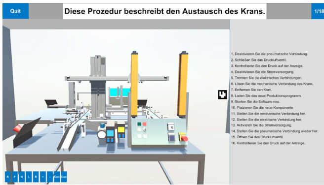
Fig. 4. Instruction provider that represents the procedure on a three-dimensional machine model.
