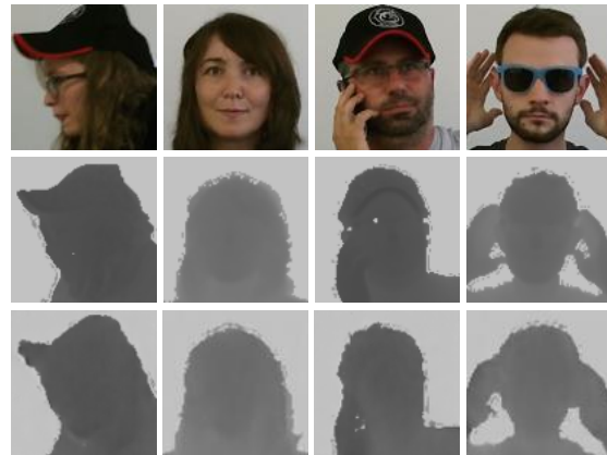
Figure 1. Examples of the RGB face images (first row), ground-truth depth images (second row), and in the last row the depth maps estimated by the proposed model. Not only are generated face images visually realistic and pleasant, but they also preserve discriminative features for the face verification task.
