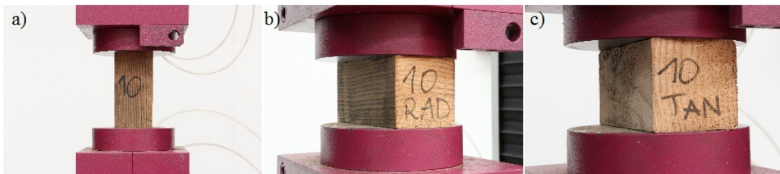
Figure 4: A timber sample under compression test (before the test). a) Longitudinal compression. b) Radial compression. c) Tangential compression.
