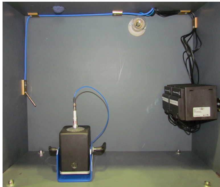
Figure 3. Experimental test rig with climatic chamber and mini shaker
