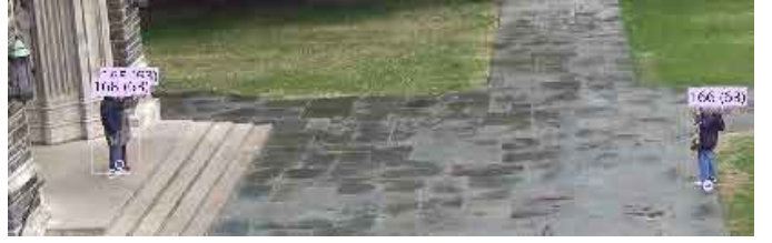
Fig. 3: One member is taking a picture of the rest of the group. Here, neither the appearance model of individual members nor their motion holds constant. The first fails because of mutual occlusion of members, the second because of a member’s independent motion.
