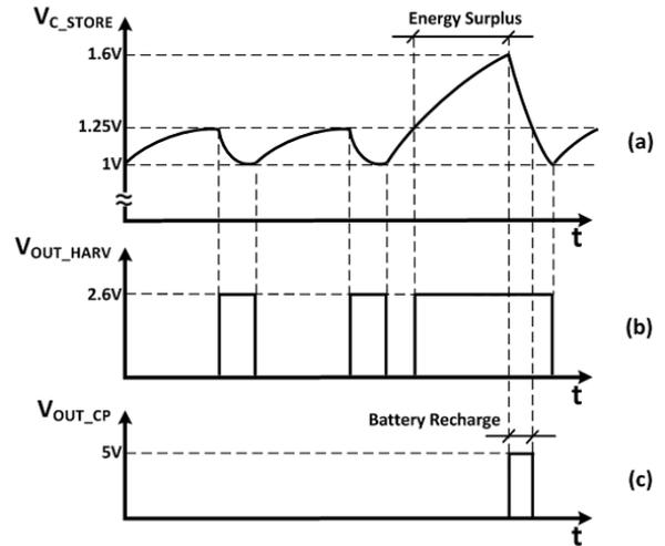
Fig. 4. Qualitative schematization of the basic operating principle of the implemented power management system through key waveforms (time axis not in scale). a) Voltage across  $C_{STORE}$ ; b) RF-DC converter output voltage; c) Charge pump output voltage.
