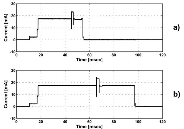
Fig. 7. Current consumption of the ED when in Advertising and Link Mode. a) Current profile of the transmission of ADV\_PKT\_SHORT and LINK\_PKT during the first stage of the advertising mode and the normal operation in Link Mode; b) Current profile of the transmission of ADV\_PKT\_FULL during the final stage of the connection procedure in Advertising Mode.
