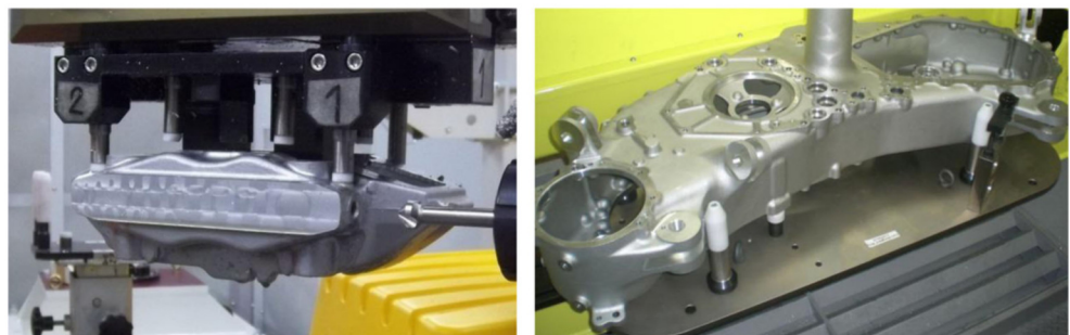
Fig. 1 Product clamping for a part-on-robot configuration ( left ) and tool-on-robot configuration ( right ) (courtesy SIR SpA–Italy)
