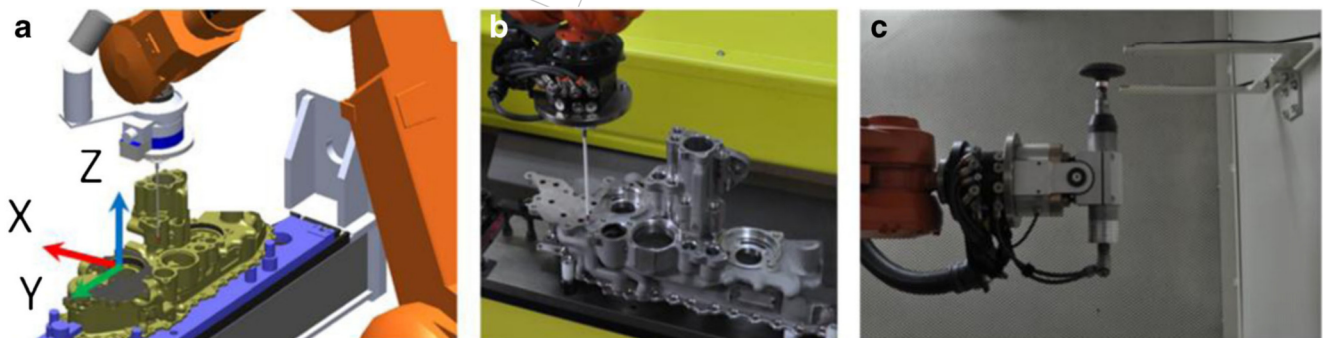
Fig. 9 OLP (a) of online workpiece (b) and tool calibration (c)
