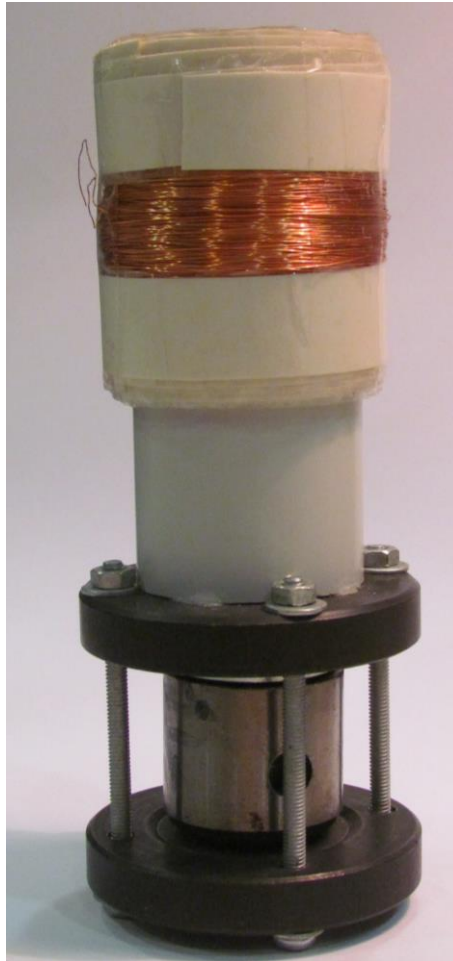
Figure 9 Harvester prototype on the vibrating table
