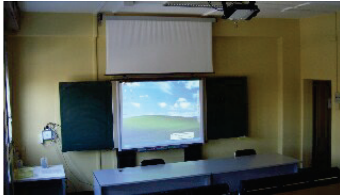
Fig. 4. A typical digital whiteboard installation: note the presence of the traditional blackboard and the installation of the PC fixed to the wall on the left
