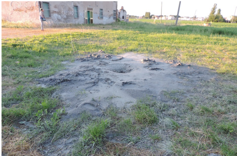
Fig. 8. Sand boil which took place on 31/05/2014 at the outskirts of Bondeno (Ferrara Province). Note the similarity with the sand boils in Fig. 2.
