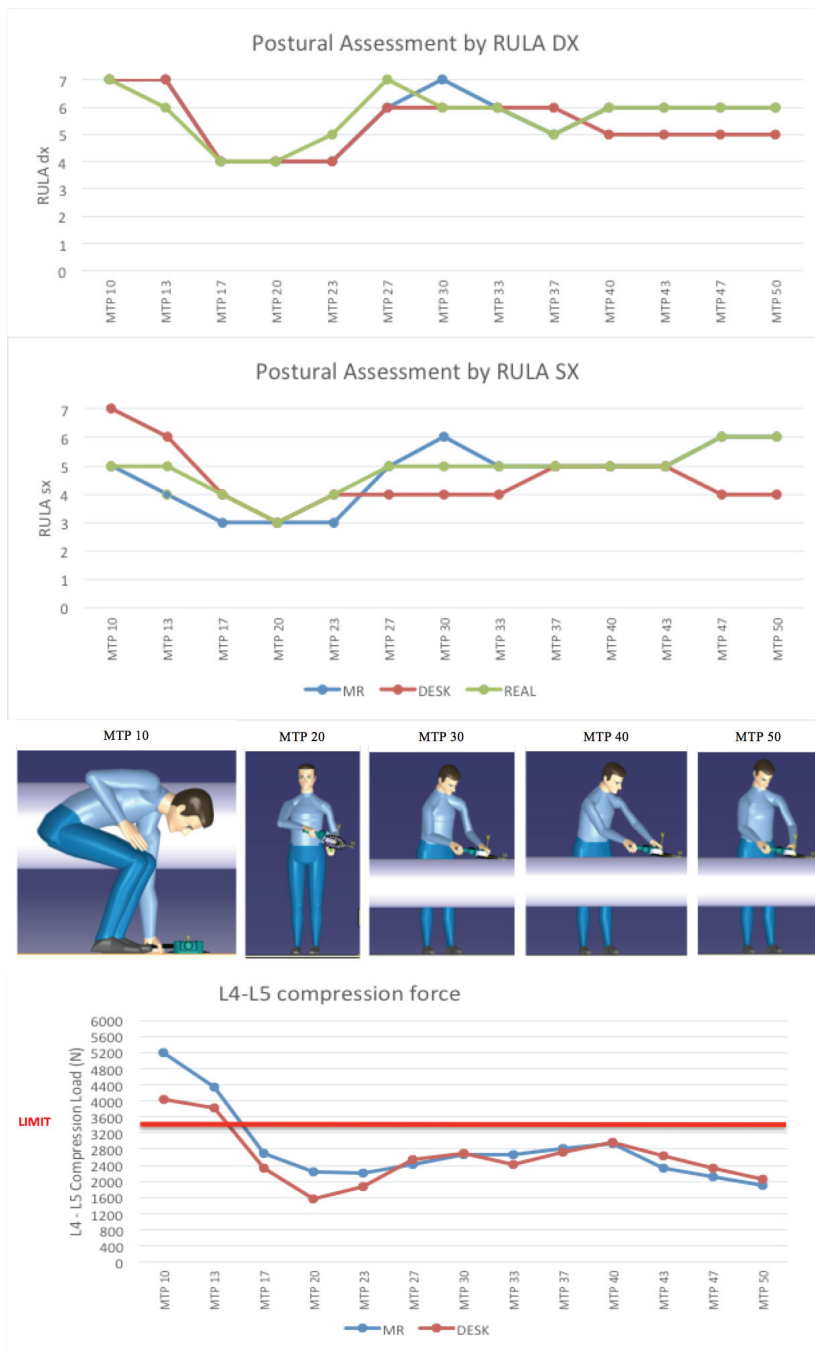
Fig. 3. Example of simulation results for the case study: comparison among different simulation modality (based on mixed reality immersive environment, desktop-based and observation of real users)
