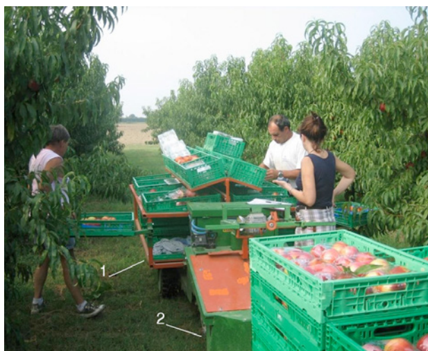
Fig. 1 - Platform for sorting, harvesting and packing fruits. 1, self-moving working platform; 2, farm cart for transport.
