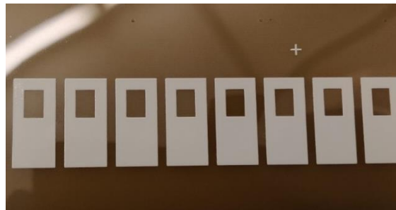
Figure 2.25: Screen-printed microfluidic pools on top of PET substrate.
