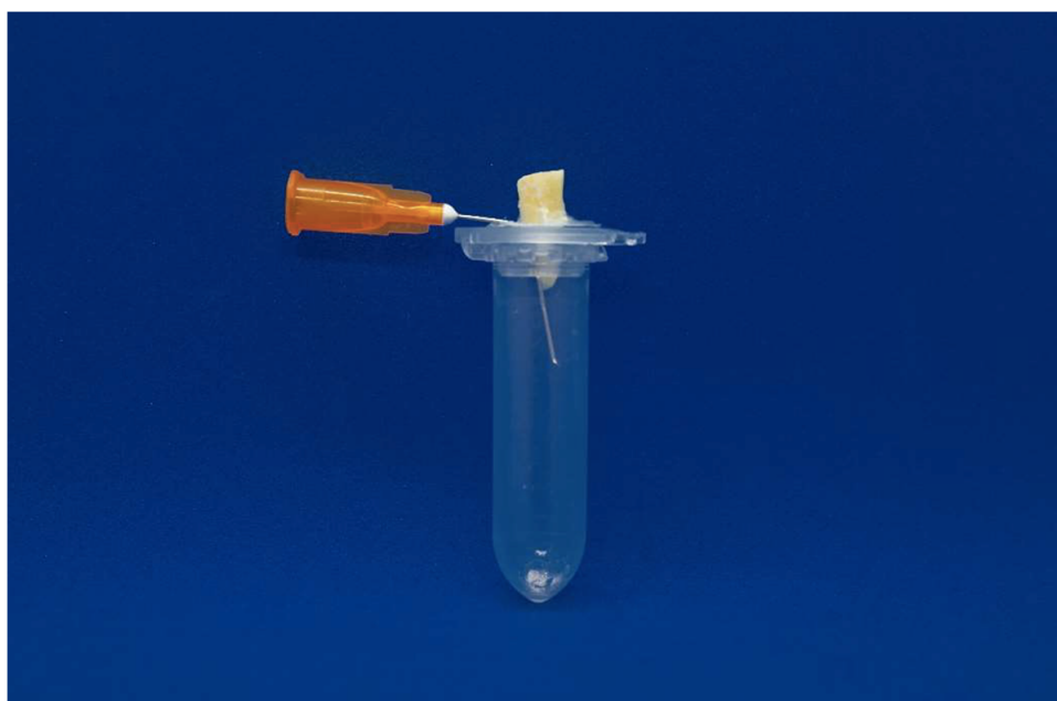
Figure 1. Eppendorf tube with root sample and 25 G needle fixed to vial stopper to balance internal and external pressures.
