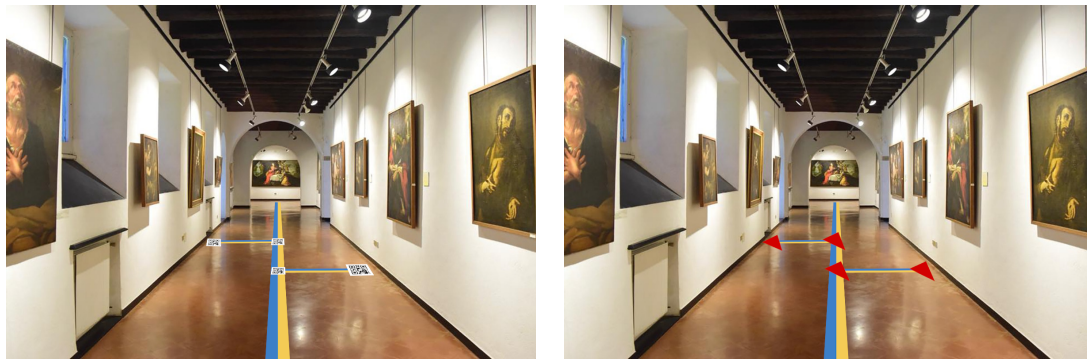
Figure 1. A possible installation of the ARIANNA system in a museum, with QRcode (a) and visual landmarks (b).
