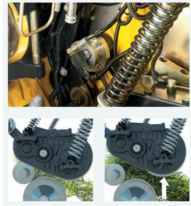
FIGURE 4 | Yield monitoring system based on continuously measuring of the opening of the feedrolls proposed by New Holland in his FR series forage harvesters. (New Holland 2024a, 2024b)
