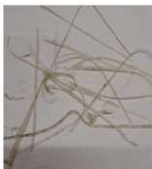
Fig. 17: Blended sample 50:50 (sheet D : virgin PC)
