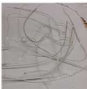
Fig. 13: Blended sample 5:95 (sheet D : virgin PC)
