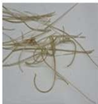
Fig. 11: Blended sample 20:80 (sheet C : virgin PC)
