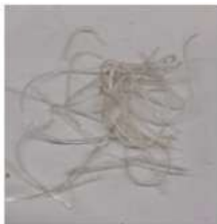
Fig. 15: Blended sample 20:80 (sheet D : virgin PC)
