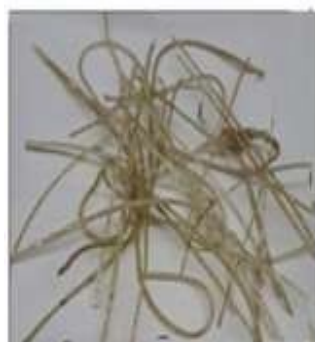
Figure 12: Blended sample 30:70 (sheet C : virgin PC)
