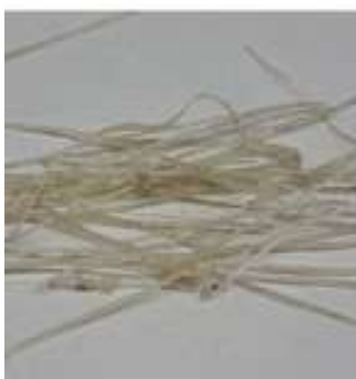
Fig. 10: Blended sample 10:90 (sheet C : virgin PC)
