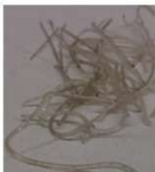
Fig. 16: Blended sample 30:70 (sheet D : virgin PC)
