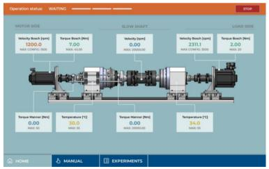
Figure 3. HMI homepage as designed - optimized solution.
