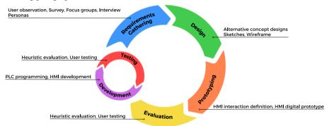
Figure 1. UX-driven cycle for HMI design.
