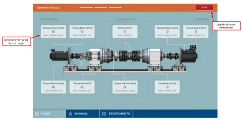
Figure 5. HMI homepage on TwinCAT HMI - as developed.
