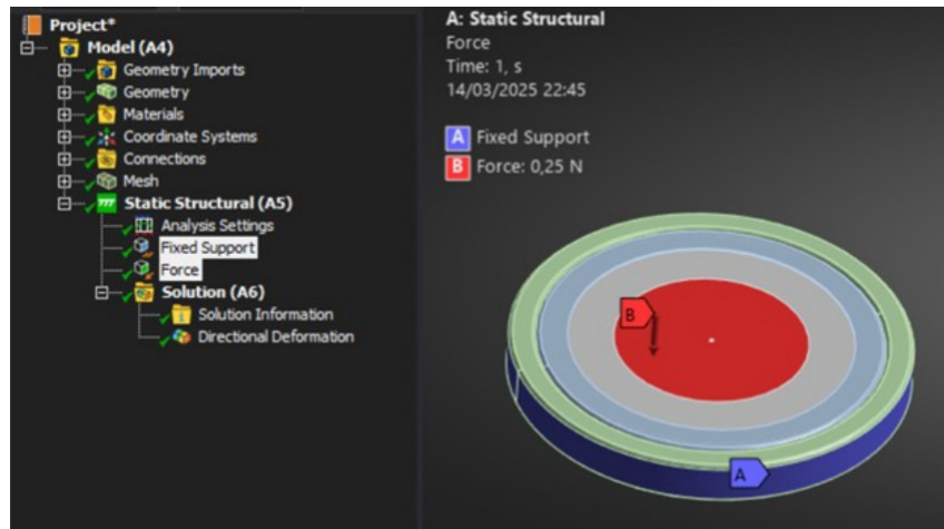
Figure 4.8: Simulation setup in Ansys environment suitable to devise the parameters of the Littmann Master Cardiology commercial diaphragm.
