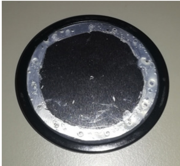
(b) Central disc in aluminum alloy plus suspension in silicone plus outer ring of Littmann Master Cardiology stethoscope.
