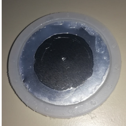
Figure 5.17: Optimized membrane composed of central disc in aluminum alloy and outer ring and suspension in silicone.
