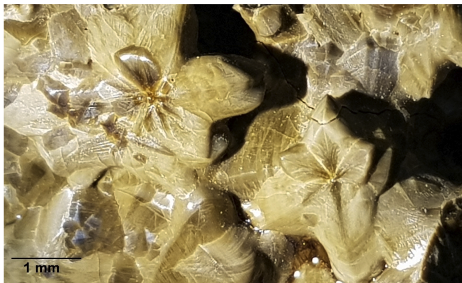
Fig. 1. Synthetic diopside product showing radiating aggregates resembling those observed in the natural rock symplectites.
