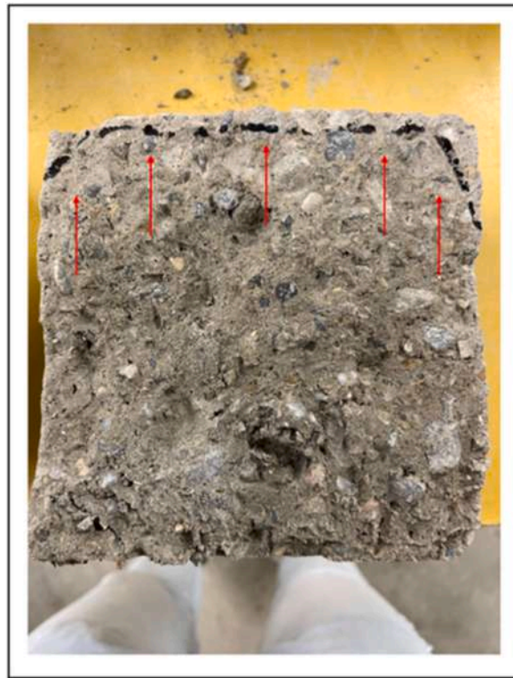
Fig. 6. Example of visible waterfront in SE1 after pressure exposure.
