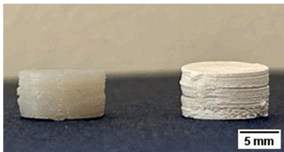
Fig. 3. Test specimen of 1M (left) before immersion and (right) after 4 weeks of degradation in H_2O . Scale bar: 5 mm.
