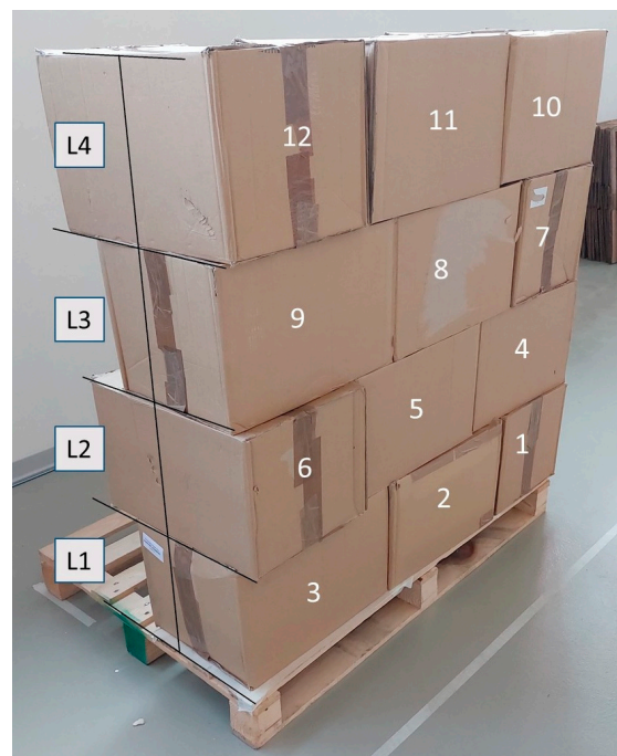
Figure 7. Deposit sequence of the boxes on the four levels (L1, L2, L3, L4) on the deposit pallet.
