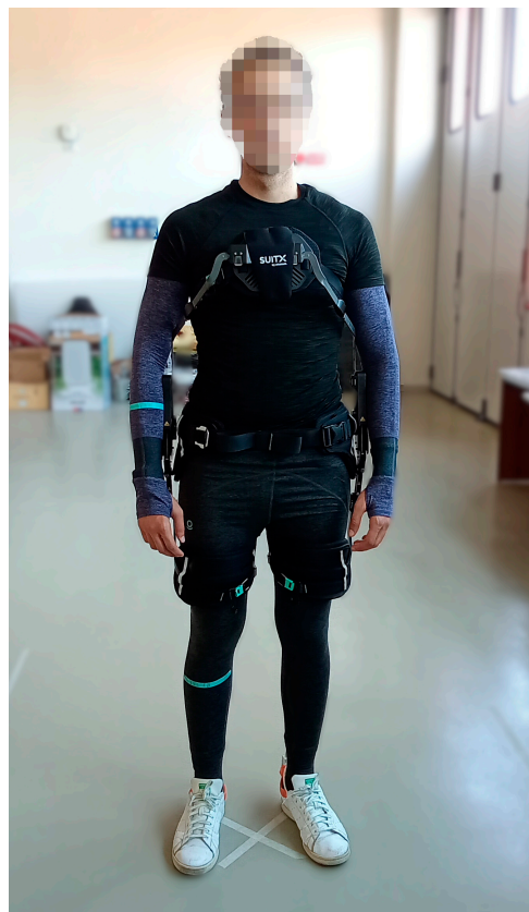
Figure 5. The technological setup with the motion capture garment, sensorized baropodometric insoles, sensorized wristband, and passive back-support exoskeleton IX BACK AIR.
