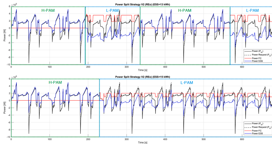
Fig. 12. Power split employing V2 strategy for 5 laps of Magny-Cours circuit for 13 (top), 15 (bottom) kWh ESS.
