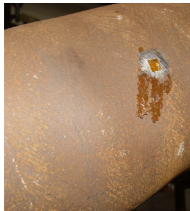
(b) Shear lines on the surface of the compression brace of specimen CFST-6
