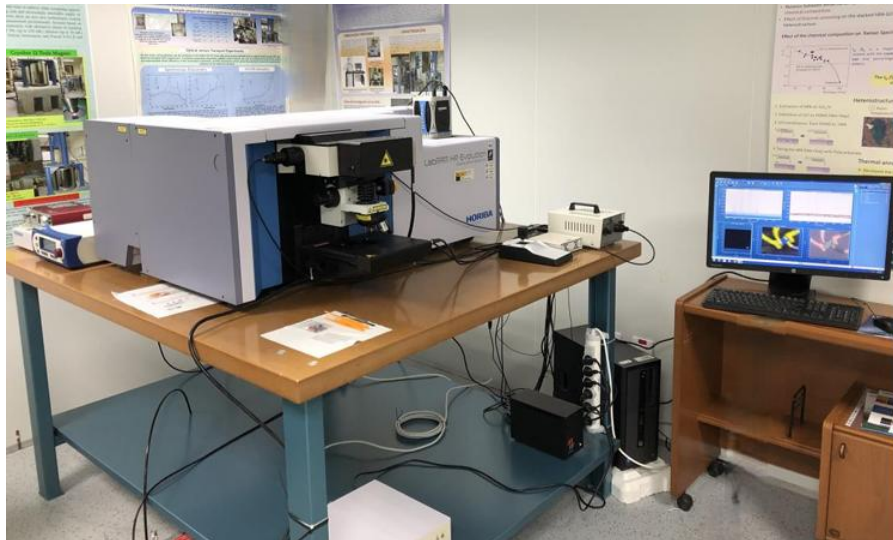
Figure 5-5. Raman spectroscopy used to assess the quality of graphene, providing information on layer number, structural defects, and crystallinity through characteristic vibrational modes.
