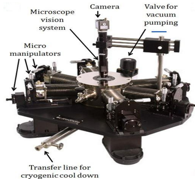
Figure 5-9. Probe station setup used for performing electrical measurements on the fabricated graphene device, showing the arrangement of probes, contacts, and instrumentation for accurate characterization of device performance.
