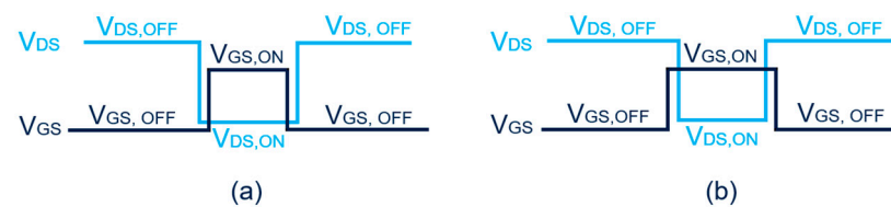
Figure 7. Waveforms corresponding to (a) soft-switching mode (i.e., in which the DUT is turned ON/OFF at 0 V drain voltage) and (b) hard-switching mode (i.e., in which the DUT is turned ON/OFF at V_{DS} = V_{DS,off} ).
