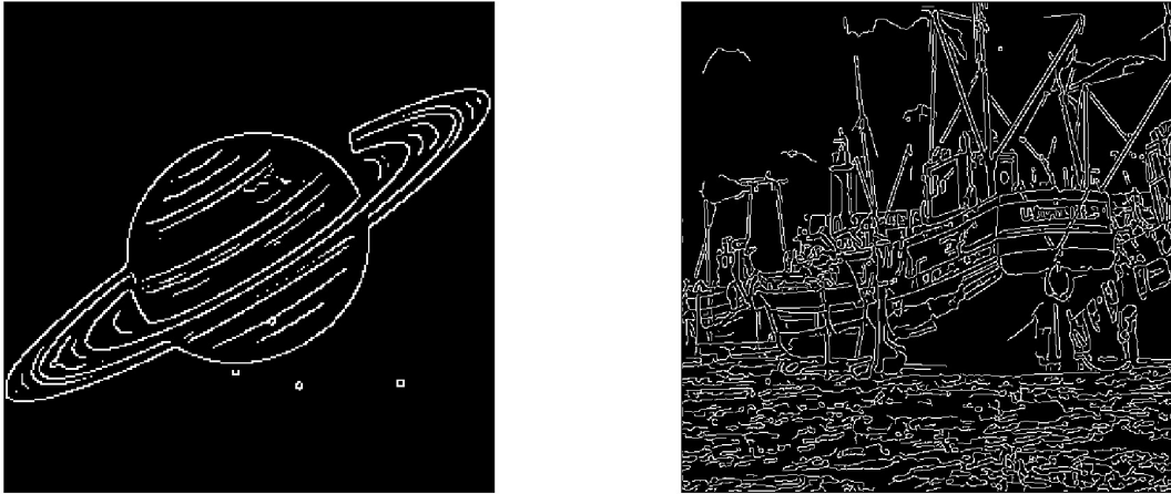
Figure 10: The results of the Canny algorithm applied to the two images used for the tests.
