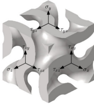
Figure 4 Representation of stress components applied to the periodic unit cell
