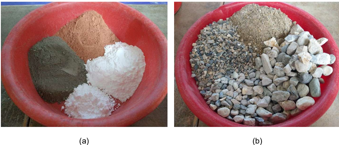
Figure 8. Solid components of the concrete mix: a) \text{LC}^3 binder with CEMI in grey, calcined clay in red, limestone in white and gypsum in white-smaller quantity, b) four aggregate fractions.
