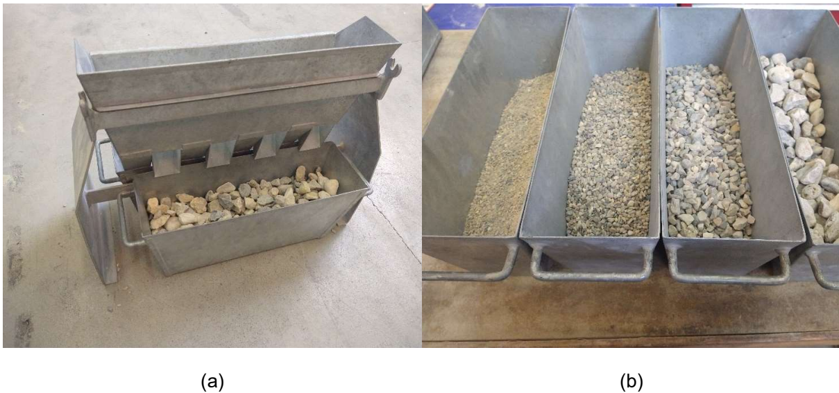
Figure 7. Representative sampling of the aggregate fractions prior to test: a) sample splitter, b) sampled fractions.
