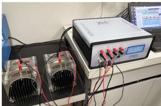
Figure 11. Experimental set-up as per the ASTM C1202-12 for the Rapid Chloride ions Penetration Test (RCPT).
