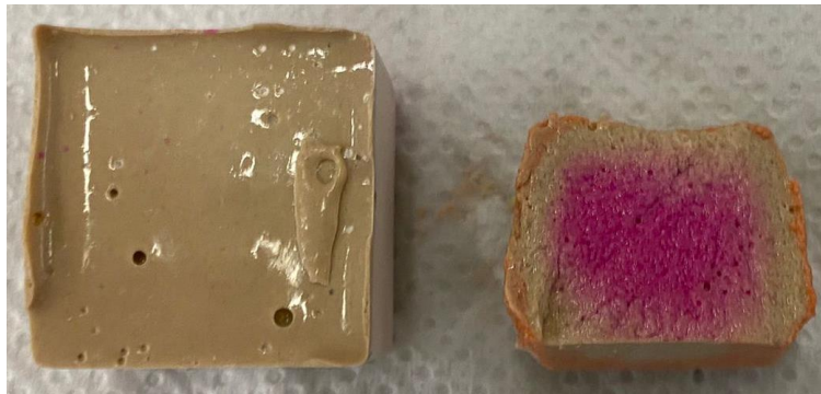
Fig.3-13 Picture of GPO sprayed with phenol. 1% after immersion in HNO 3 2.5N.
