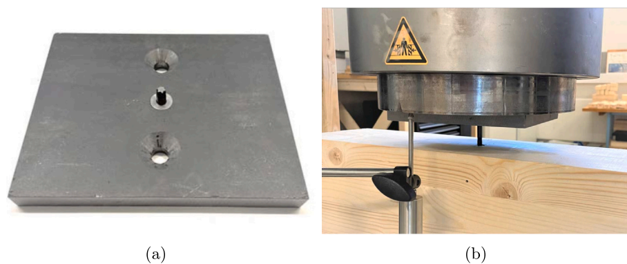
Fig. 5. Setup of specimen with height 540 mm in ZwickRoell Z1200-Steel plate used for Torx tests — Setup of Torx test.
