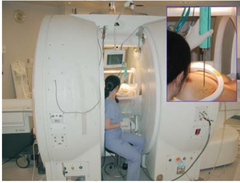
Figure 3. Positioning for prone freehand vacuum core biopsy. The patient lies on an open breast coil (Custom OBC, MRI-Devices/Invivo Inc, Waukesha, WI) in the 0.5 T vertically open scanner (Signa-SP, GE Healthcare, Milwaukee, WI).
