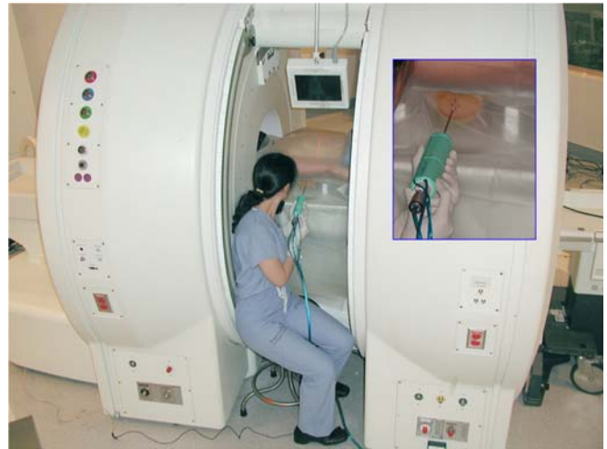
Figure 1. Positioning for prone freehand vacuum core biopsy. The patient lies on an open breast coil (Custom OBC, MRI-Devices/Invivo Inc, Waukesha, WI) in the 0.5 T vertically open scanner (Signa-SP, GE Healthcare, Milwaukee, WI).
