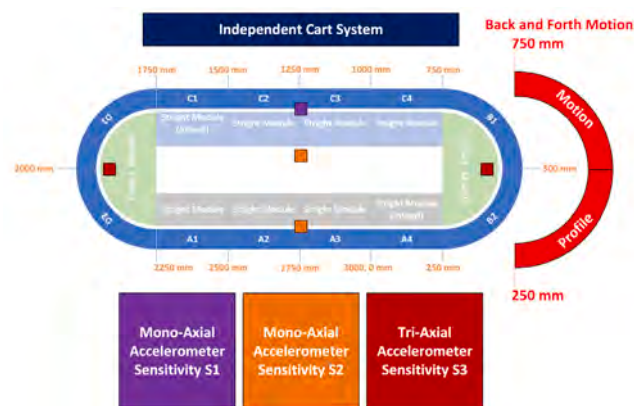
Fig. 5. The topological schematic of the experimental Independent Cart System (ICS) is presented, featuring annotated dimensions, sensor locations, and the motion profile. The oval-shaped track comprised straight (C1–C4, A1–A4) and curved (D1–D2, B1–B2) modules, facilitating a closed loop. Colored squares indicate accelerometer placements: S1 and S2 represent the mono-axial sensor sensitivities on the straight sections, whereas S3 denotes the tri-axial sensor sensitivity situated on the curved section. The dimension labels specify the distances between the key module boundaries (in mm). The red arc on the right delineates the 500 mm back-and-forth reversal zone employed during testing to induce bidirectional motion.
