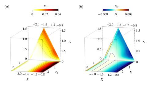
FIGURE 13. Production terms  $P_{11}$  (a) and  $P_{22}$  (b) in the  $(X, r_x, r_z)$ -space for  $r_y = 0$  and Y = 0.64. Black contour lines indicate increments of 0.005.
