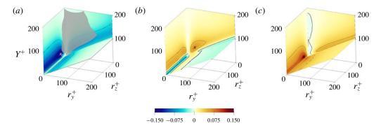
FIGURE 3. Colour plot of  $\Pi_{11}^+$  (a),  $\Pi_{22}^+$  (b) and  $\Pi_{33}^+$  (c) on the bounding planes  $r_y^+=0$ ,  $r_z^+=0$  and  $Y^+=r_y^+/2$ . The contour lines increment is 0.04, with level zero indicated by a thick line. The two symbols identify the positions of the maxima of  $\Pi_{ij}$  (cross) and  $P_{ij}$  (circle). The isosurface in (a) corresponds to  $\Pi_{22}/\Pi_{11}=-0.5$  (or equivalently  $\Pi_{33}/\Pi_{11}=-0.5$ ), with  $\Pi_{22}/\Pi_{11}<-0.5$  for smaller scales.
