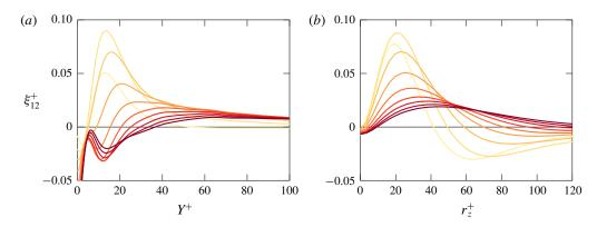
FIGURE 5. Source term  $\xi_{12}$  in the  $r_y = 0$  plane. (a)  $\xi_{12}^+$  versus  $Y^+$  for different  $r_z^+ = (10:100)$ . (b)  $\xi_{12}^+$  versus  $r_z^+$  for different  $Y^+ = (10:5:50)$ . Line colours encode the value of the parameter, which increases from yellow (light) to red (dark).
