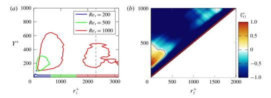
FIGURE 9. (a) Contour  $\xi_{11} = 0$  for  $Re_{\tau} = 200$ , 500 and 1000 in the  $(r_z, Y)$  plane at  $r_x = r_y = 0$ . (b) Colour map of  $\xi_{11}$  at  $Re_{\tau} = 1000$  in the  $(r_y, Y)$  plane for  $r_x = 0$  and  $r_z^+ = 2300$ , i.e. for the plane shown in the left panel (vertical dashed line) which crosses the large-scale  $\xi_{11}$  maximum at  $Re_{\tau} = 1000$ .
