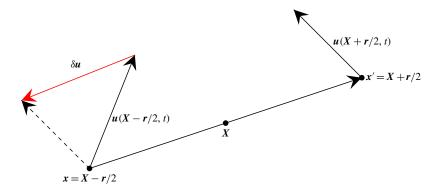
FIGURE 2. Sketch of the quantities involved in the definition of the second-order structure function. x = X - r/2 and x' = X + r/2 are the two points across which the velocity increment  $\delta u$  is computed.
