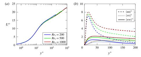
FIGURE 8. Profile of (a) mean velocity and (b) velocity fluctuation variance at  $Re_{\tau} = 200$ , 500 and 1000. For validation, in both panels data from Lee & Moser (2015) at  $Re_{\tau} = 1000$  are also plotted with a thin black line connecting open symbols, which is nearly perfectly overlapping.
