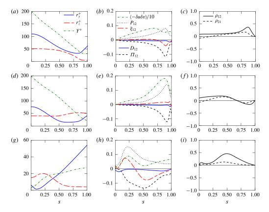
FIGURE 6. Field lines of the flux vector for  $\langle -\delta u \delta v \rangle$ . (a-c) Set I; (d-f) Set II; (g-i) Set IV. (a,d,g) Evolution of the values of Y (-----, dark green),  $r_y$  (-----, blue),  $r_z$  (-----, red), along a representative field line as a function of its dimensionless arc length s. (b,e,h) Values of  $\langle -\delta u \delta v \rangle / 10$  (-----, dark green),  $\xi_{12}$  (----, red),  $P_{12}$  (-----),  $P_{12}$  (-----) along the line.
