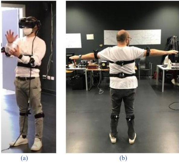
Figure 3 (a) shows the complete sensors' setup for the virtual simulation; (b) shows the disposition of the Vive Trackers according to the ErgoForce user profile within the XRErgo software.
