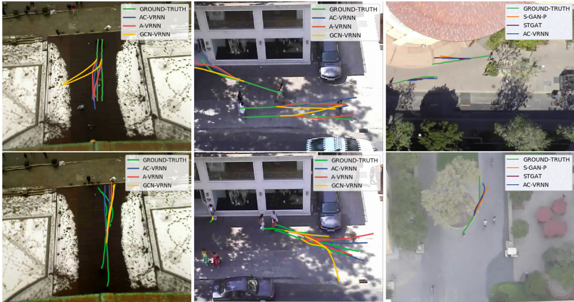
Fig. 3. Illustration of predicted trajectories using AC-VRNN, baselines and competitive methods on Eth (left) and Zara1 (middle) scenes of ETH and UCY datasets and gates_0 and deathCircle_1 of SDD (right).
